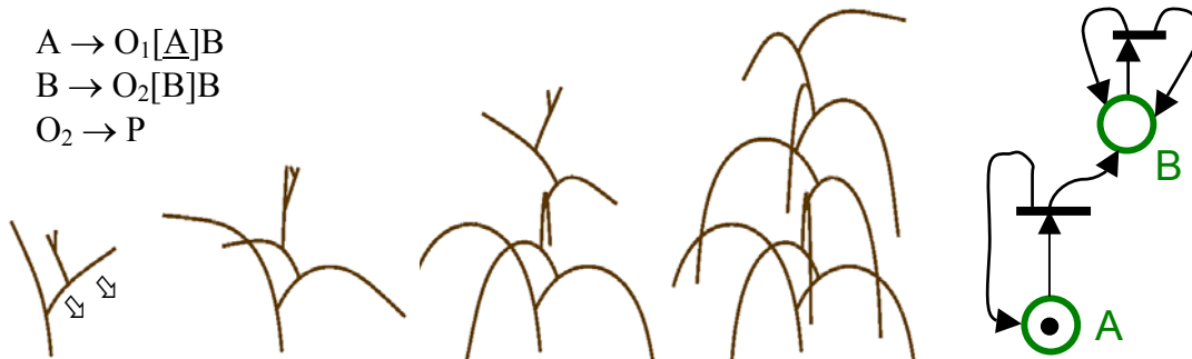
Figure 25. L-system productions, four stages of simulated development, and Petri net for Champagnat's model. The arrows in the first drawing indicate the direction of shoot reorientation.
