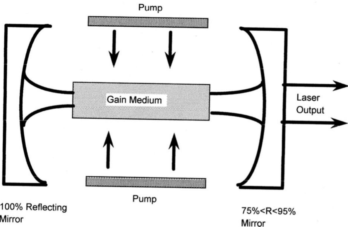
2 MIRRORS to contain the light. One is partially reflecting to let light out to be used.
