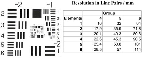
Figure 6, USAF Resolution Test Pattern
