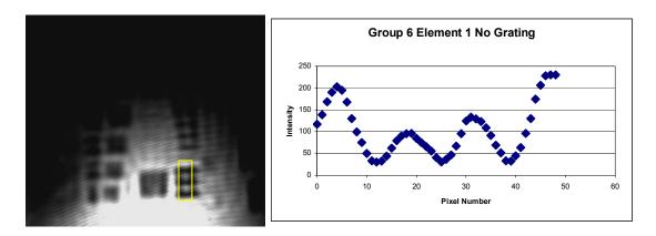
Figure 12 Group 6 Element 1 Without Diffuser Plate
