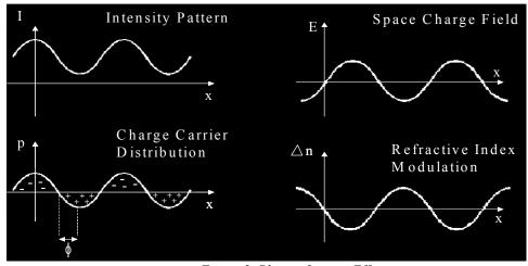
Figure 2, Photorefractive Effect
