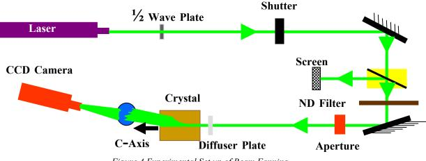
Figure 4 Experimental Set up of Beam Fanning
